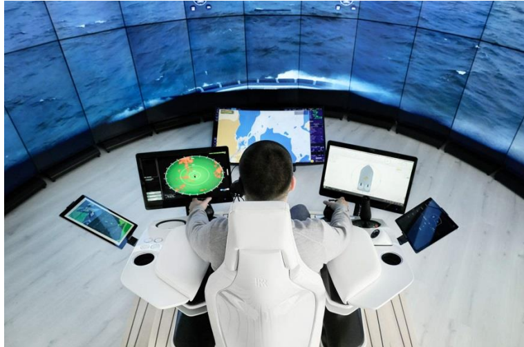
Fig.2. Remote operation station for autonomous ship, note nautical chart displayed [7]
